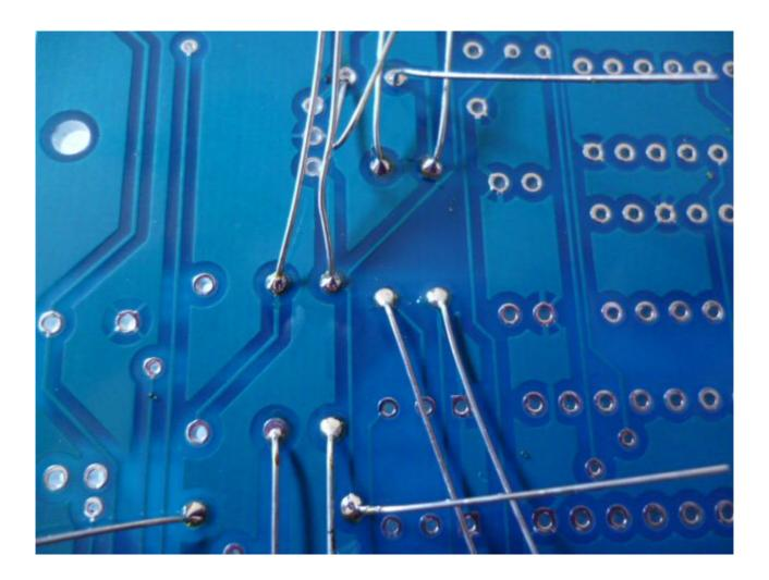
5. Now insert multilayer capacitors, 100nF and R12, R PACK. Solder it.
