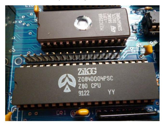
The quartz window of the EPROM can be opened for showing student to see the silicon chip.
