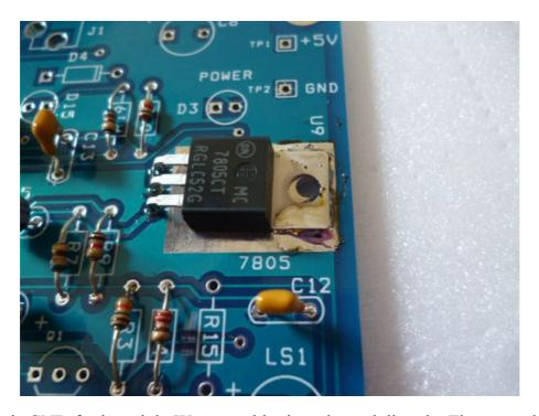
The TAP pin is GND for heatsink. We can solder it to the pad directly. The ground plan will be heatsink of the voltage regulator. You can tighten the TAP to the PCB with M3 nut and washer as well.
