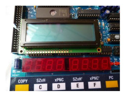
Your first computer shall look like this when powers it on. For LCD, adjust R18 to make the first line appears.
