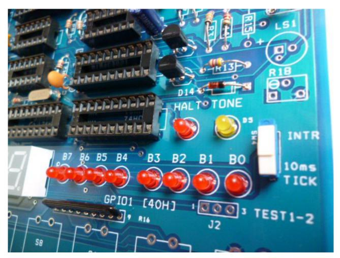
Again SW4 is not easy to stand, just solder one pin, then adjust the position with finger while soldering.
