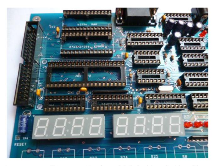
For seven segment LED, we may solder only one pin beforehand. Then check the position, both should be line up on the same level.
