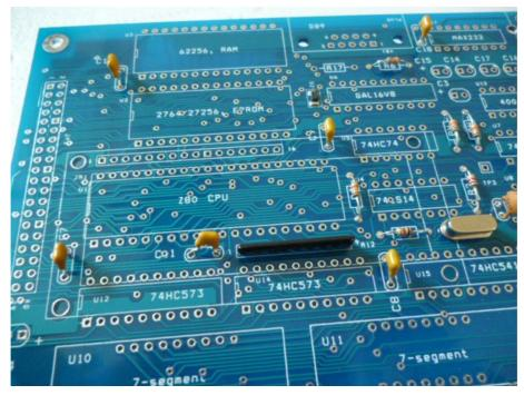
6. Insert R16, R PACK. Pin 1 of R pack is a dot point! Soldering R pack many need your finger to press it.
