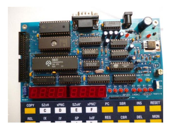
Pin 1 has indicator on the IC chips. Shown Zilog Z80 CPU and monitor EPROM, 27C256.
