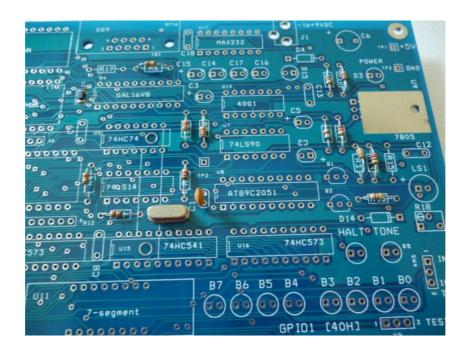
For resistors and capacitors, we can bend the legs to make it in place. So we can solder it easily.
