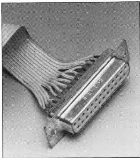
Fig. 15. Centronics printer cable details.
