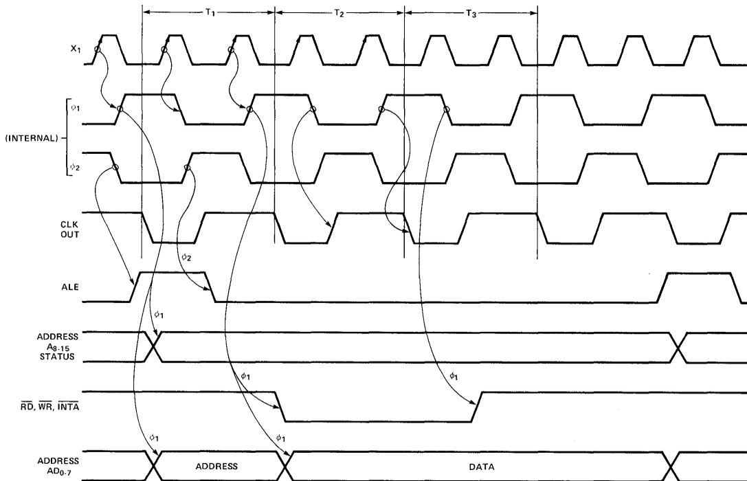
**Figure 14. Clock In ( $X_1$ ) to Output Relationship**
