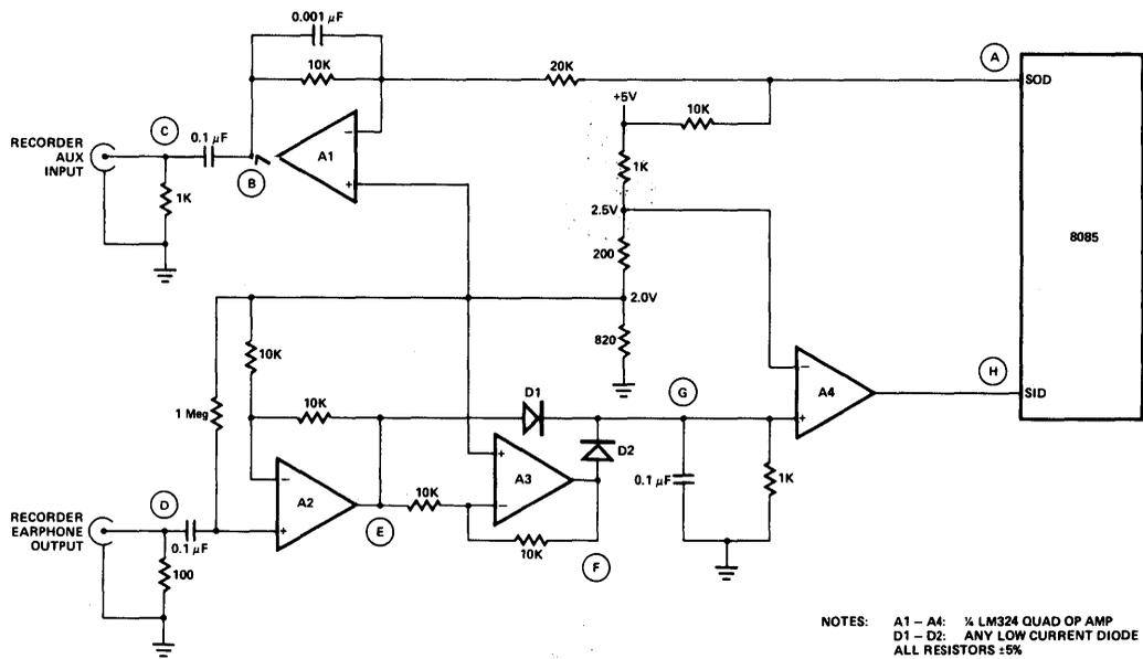
Figure 26. One Chip Magnetic Tape Interface Schematic
