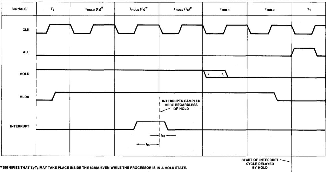
**FIGURE 2-21 HOLD VS INTERRUPT — NON HALT**
