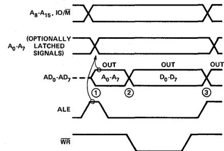
The timing of the WRITE CYCLE is identical to the MCS-85 READ CYCLE with the exception of the AD<sub>0</sub>-AD<sub>7</sub> lines. At the beginning of the cycle ①, the low order eight bits of address are on AD<sub>0</sub>-AD<sub>7</sub>. After ALE drops, the eight bits of data ② are put on AD<sub>0</sub>-AD<sub>7</sub>. They are removed ③ at the end of the WRITE CYCLE, in anticipation of the next data transfer.
