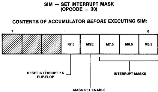
**FIGURE 2-4 INTERRUPT MASKS SET USING SIM INSTRUCTION**
