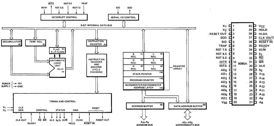
Figure 1. 8085A CPU Functional Block Diagram
