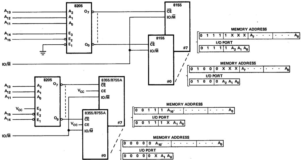
**FIGURE 3-1D SEPARATE CHIP ENABLES FOR I/O AND MEMORY**
