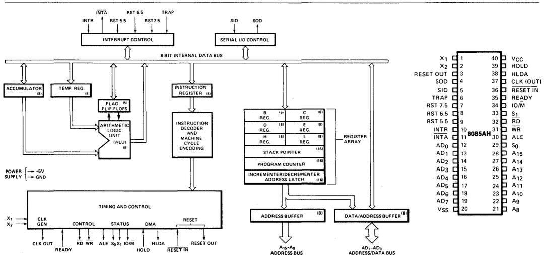
Figure 1. 8085AH CPU Functional Block Diagram
