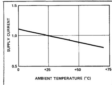
**Typical Supply Current vs. Temperature, Normalized**<sup>[3]</sup>
