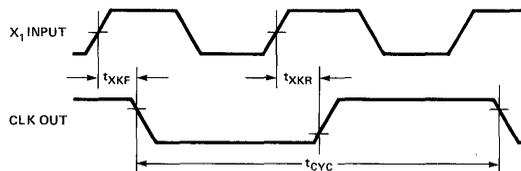
**Figure 15. 8085A-2 Clock In/Clock Out Timing**
