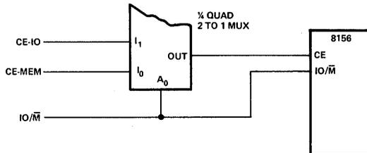
**FIGURE 3-1 MCS-85™ PERIPHERALS WITH I/O MAPPED I/O**
