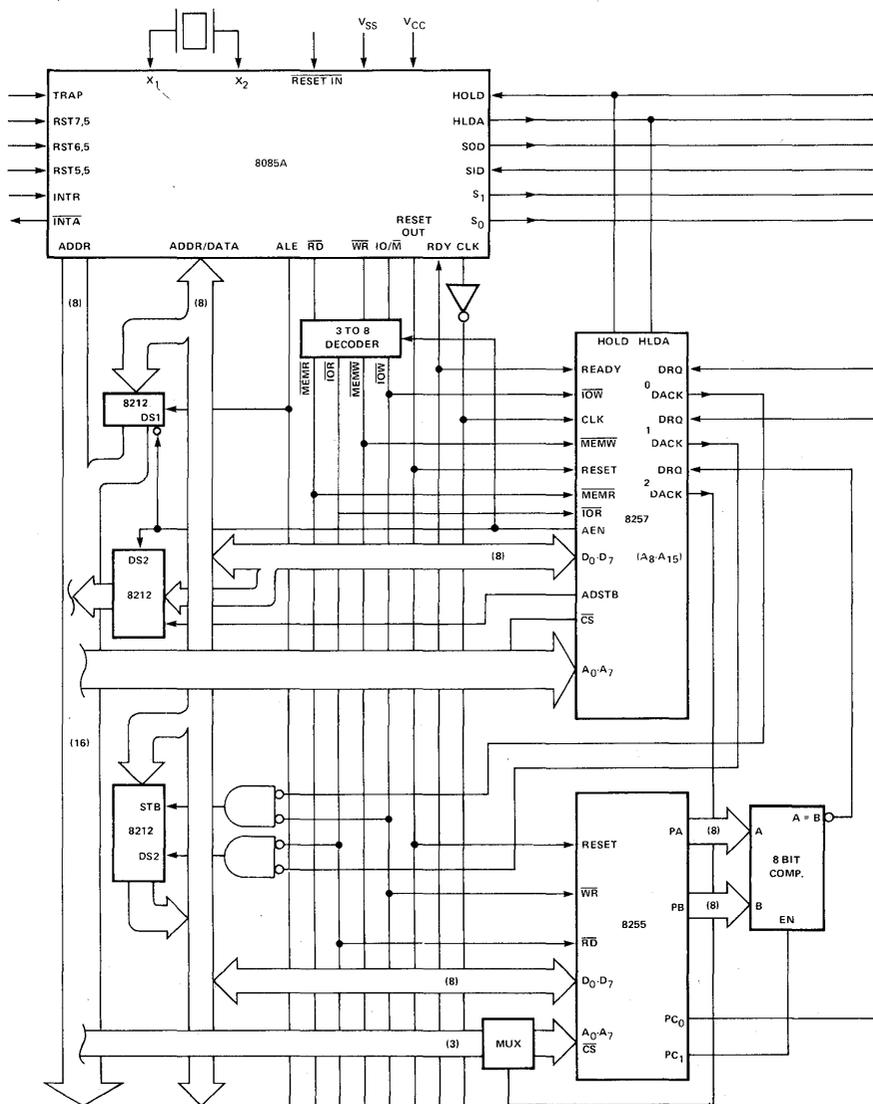
**FIGURE 4. BLOCK MOVE, BLOCK SEARCH** addition of an 8257 Direct Memory Access (DMA) controller and an 8255 Programmable Peripheral Interface (PPI) device permits block searches, high speed block moves. (2.5 μs/word).
