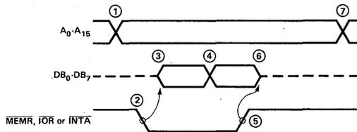
The MCS-80 first presents the address ① and shortly thereafter the control signal ②. The data bus, which was in the high impedance state, is driven by the selected device ③. The selected device eventually presents the valid data to the processor ④. The processor raises the control signal ⑤, which causes the selected device to put the data bus in the high impedance state ⑥. The processor then changes the address ⑦ for the start of the next data transfer.
