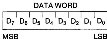
When a register or data word contains a binary number, it is necessary to establish the order in which the bits of the number are written. In the Intel 8085A, BIT 0 is referred to as the **Least Significant Bit (LSB)**, and BIT 7 (of an 8-bit number) is referred to as the **Most Significant Bit (MSB)**.
