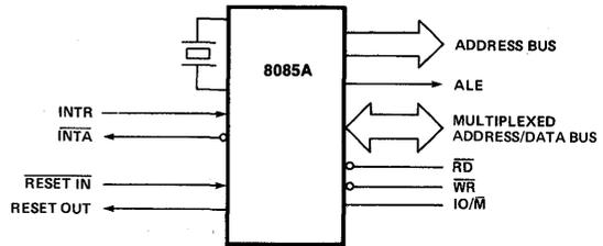
FIGURE 2-8B MCS-85™ CPU/8085A (MCS-80 COMPATIBLE FUNCTIONS)
