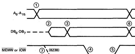
The MCS-80 first presents the address ①, then enables the data bus driver ②, and later presents the data ③. Shortly thereafter, the MCS-80 drops the control signal ④ for an interval of time and then raises the signal ⑤. The MCS-80 then changes the address ⑥ in preparation for the next data transfer. The advance write signal of the 8238 is also shown ⑦.
