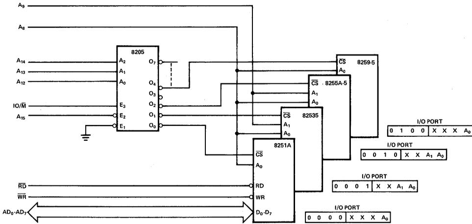
**FIGURE 3-3B DECODED CONTROLS AND LATCHED ADDRESS (MCS-80™ TYPE BUS)**
