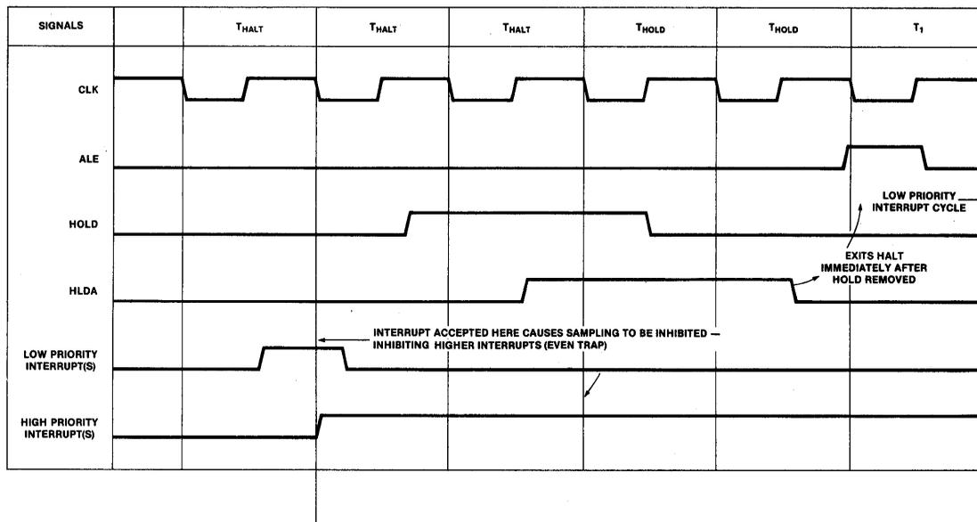
**FIGURE 2-22 8085A HOLD VS INTERRUPTS — HALT MODE**
