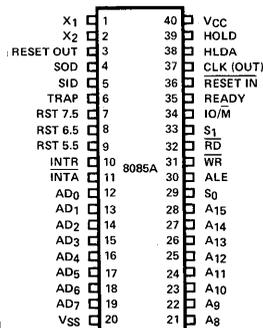
Figure 2. 8085A Pin Configuration
