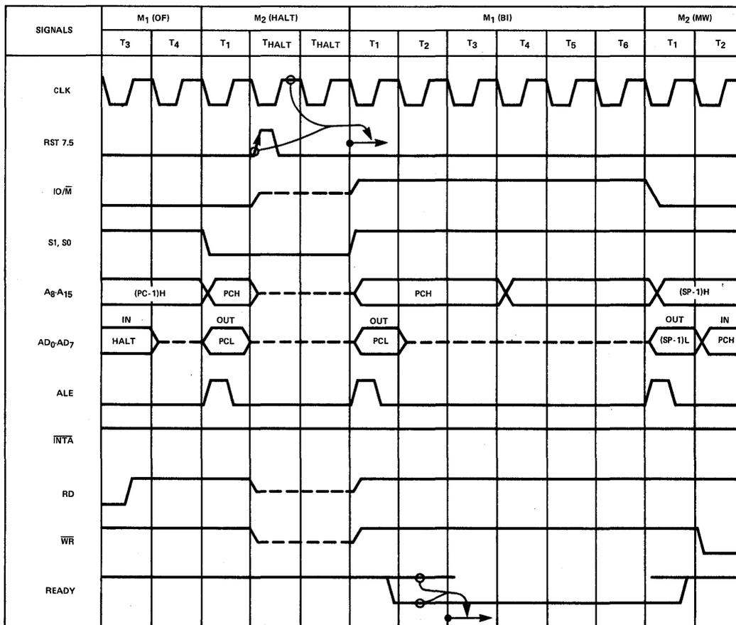
**FIGURE 2-20 HALT STATE AND BUS IDLE MACHINE CYCLE
