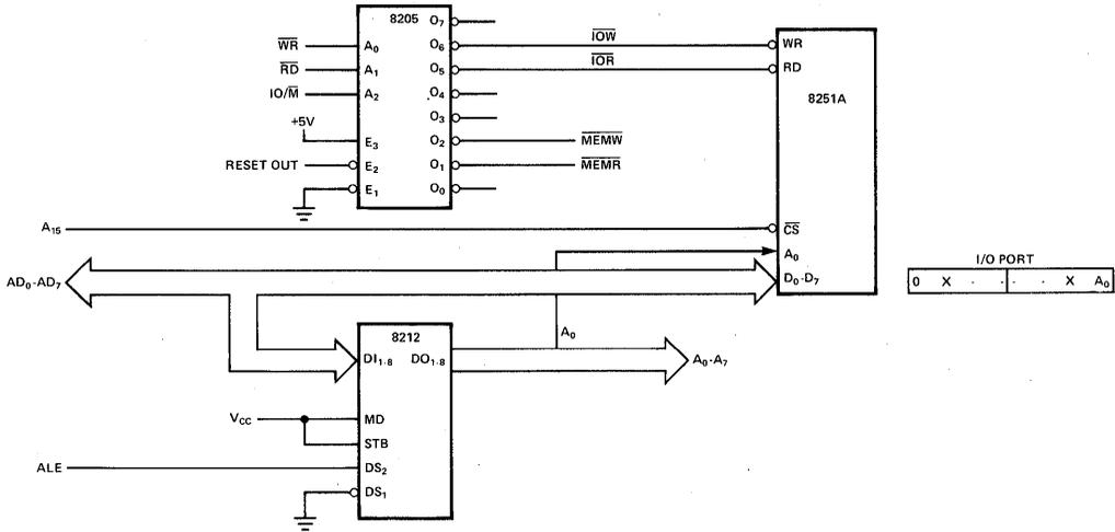
**FIGURE 3-3 MCS-80™ PERIPHERALS WITH I/O MAPPED I/O**
