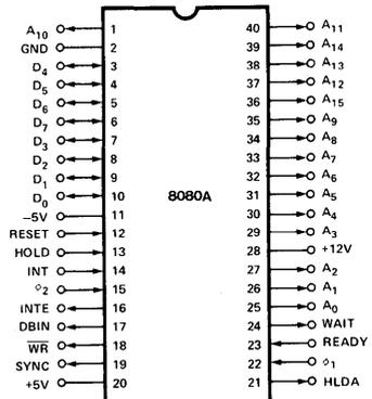
**Figure 2. Pin Configuration**
