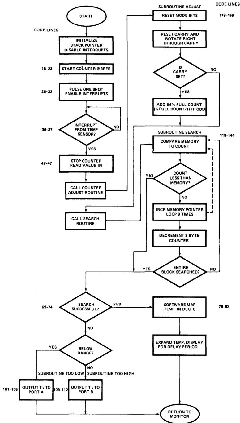
Figure 21. Temperature Sensor Flow Diagram
