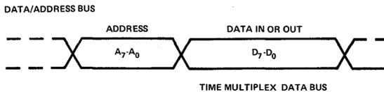
FIGURE 2-8C MULTIPLEXED BUS TIMING
