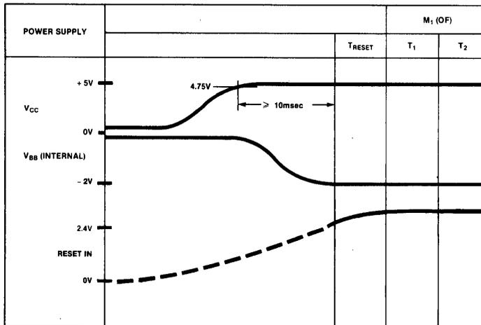
**FIGURE 2-23 POWER-ON TIMING**
