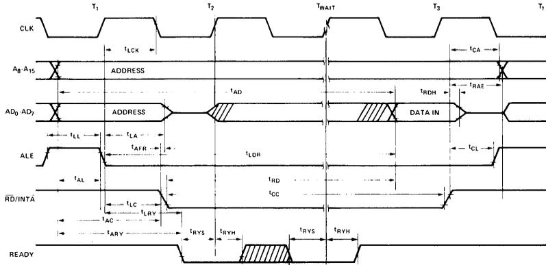
NOTE 1: READY MUST REMAIN STABLE DURING SETUP AND HOLD TIMES.
