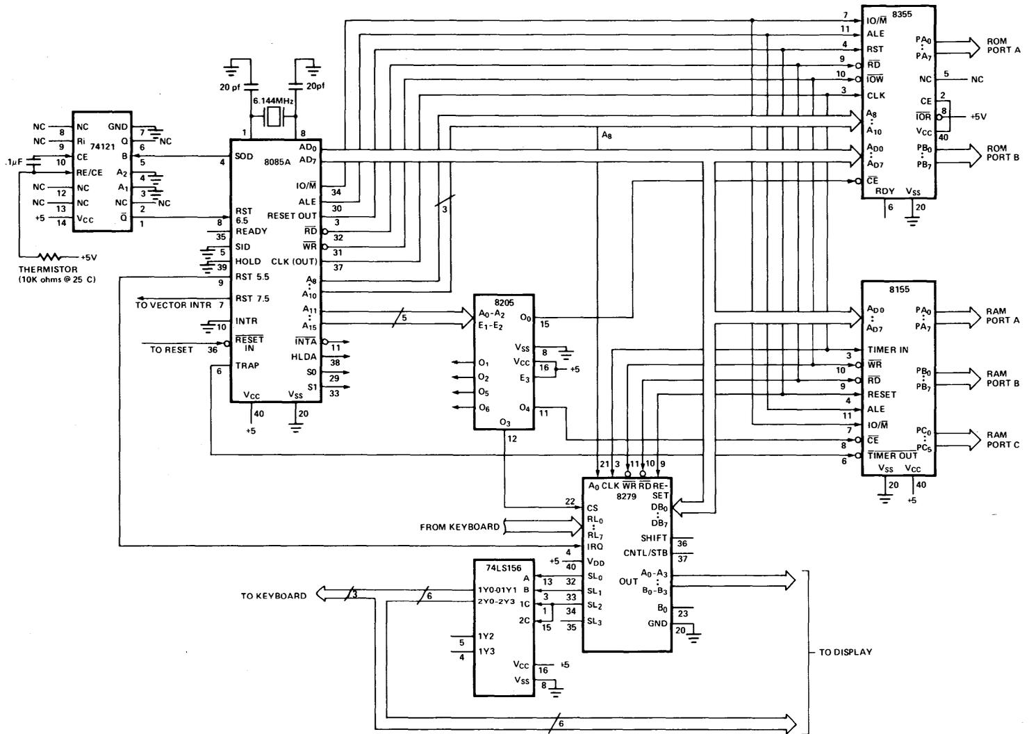
Figure 20. Detailed SDK-85 Kit with Temperature Sensor
