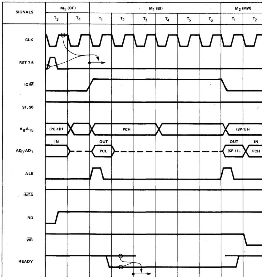
FIGURE 2-19 RST 7.5 BUS IDLE MACHINE CYCLE
