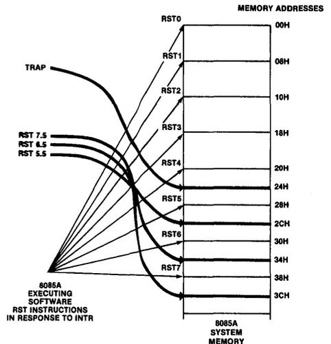
**FIGURE 2-3 8085A HARDWARE AND SOFTWARE RST BRANCH LOCATIONS**
