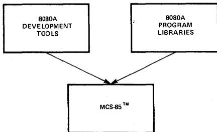
For the new microcomputer user, the software compatibility between the 8085A and the 8080A means that all of the software development tools that are available for the 8080A and all software libraries for 8080A will operate with the new design and thus save immeasurable cost in development and debug.
