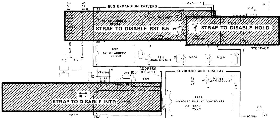
Figure 3-8 Strapping Options for Bus Expansion Control Lines
