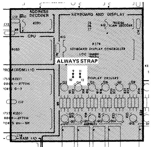
Figure 3-5 Disabling Unused Keyboard Controller Functions
