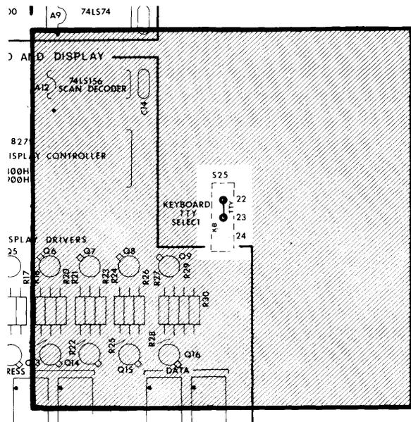
Figure 3-3 Teletypewriter Strapping Connection
