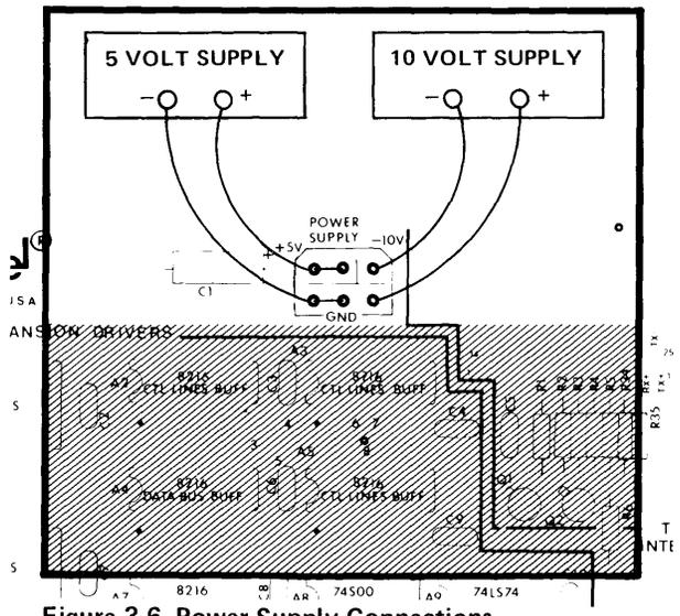
Figure 3-6 Power Supply Connections
