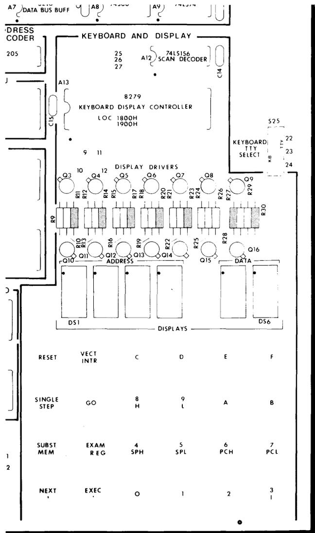
Install fourteen 2N2907 transistors in two rows. Position the seven transistors in the top row so that their indexing tabs point upward and to the left, at:
