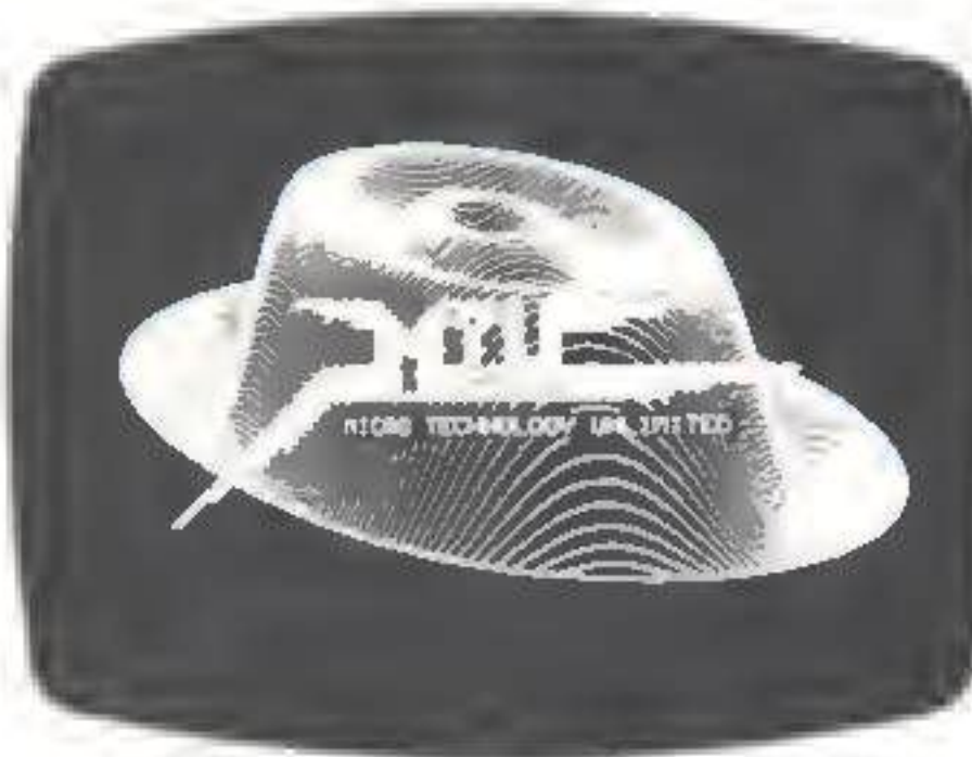
The MTU-130 displays the company's symbol in high-resolution graphics mode, which allows individual addressing of the 122,880 pixels on the screen.
