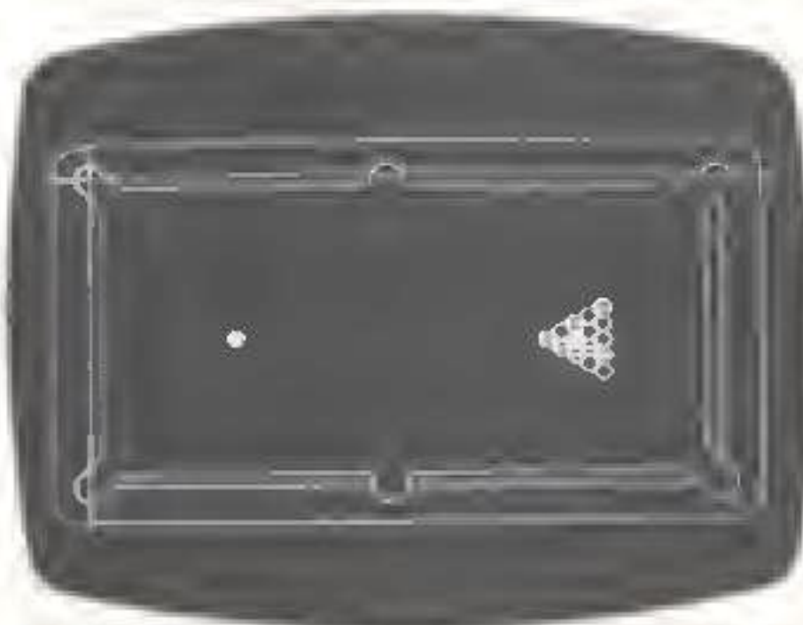
The beginning of a game of pool on the MTU-130 which combines high-resolution graphics with sound effects. The two lines which cross at the upper left pocket form the graphics cursor used in this game to specify the point at which the cue ball is aimed.
