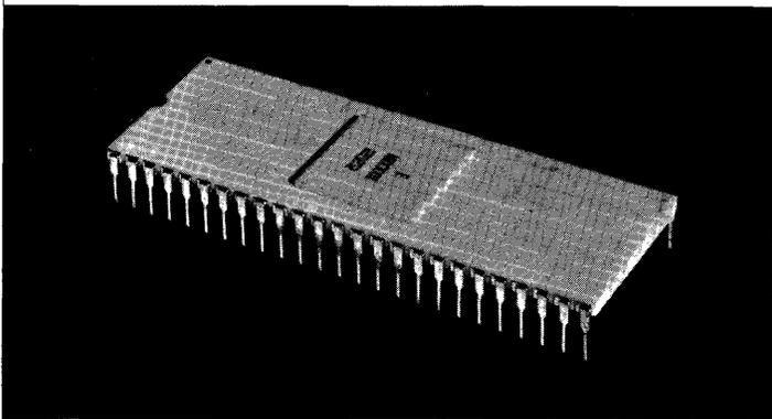
These features, combined with partitioning of the address/data bus into right and left banks, make it possible for 8-bit parallel data to be rotated or masked, to undergo arithmetic or logical operations, and then to be shifted and merged into any set of one to 8 contiguous bits at the destination—all in one 250 nanosecond cycle.
