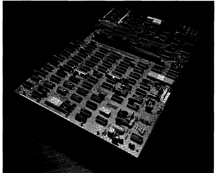
A single board PC kit for use as either a computer or intelligent terminal has been announced by Processor Technology, known as the Sol Terminal Computer, the new unit with memory and interface electronics including video display, keyboard interface, audio cassette interface, all necessary software plus the ability to accept the Processor Technology line of memory and interface modules sells for \$475 in kit form.
