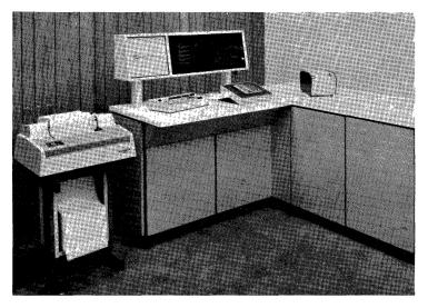
Troubleshooter 400, a new computer using the Advanced Micro Devices 9080 8-bit microcomputer is an in-circuit test system which provides complete analog and digital fault analysis to the component level on complete analog and digital fault analysis to the component level on complex PC boards plus extensive functional test capabilities, has been introduced by Zehntel, Inc.
