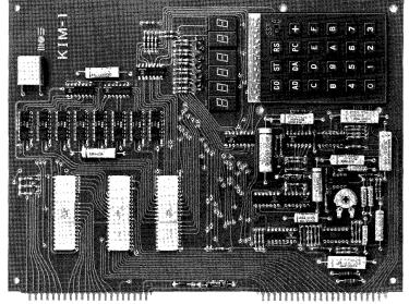
The \$245 board requires only a single power supply (5V at 1.2A) for basic operations, and a second supply (1.1A) for audio cassette operation. The KIM-1 system can be expanded to include additional memory of any variety or additional I/O capability.
