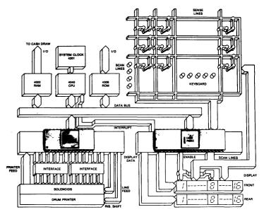
The 4269 Programmable Keyboard/Display Unit is a general-purpose interface and control unit and is configured with software and selected like a RAM-I/O unit. Each unit provides the equivalent of seven I/O ports, a RAM, a ROM, and the logic required for control and communications with man-machine interface equipment. The CPU can directly control up to four 4269 units.
