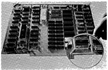
Features include an asynchronous serial receiver and transmitter for communications with TTYs and CRT terminal systems. The oncard clock allows transmission rates between 110 baud and 9600 baud and the system provides two types of interfaces, a 20 mA optically isolated current loop and a RS232C interface for use with modems or other devices using EIA levels. The microcomputer contains an 8-level vectored priority interrupt system and logic for DMA channel control.
