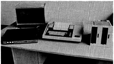
MYCRON of Oslo, Norway, is announcing the availability of MYCRO-1, a general byte-oriented 8080-based microcomputer system designed especially for dedicated applications. The functional, mechanical and electrical design is the basis for a series of machine configurations built with standard function modules.
