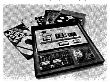
Called the MCS-80 Microcomputer System Design Kit, it provides the following components and software for only \$350: 8080A microprocessor, 8224 clock generator, 8228 system controller, 8251 programmable communications interface, 8255 programmable peripheral interface, two 8205 l-out-of-8 binary decoders, two 8708 8K EPROMs, two 8111 1K RAMs, clock crystal, PC board, connectors, all required discrete components, system monitor program, and documentation.
