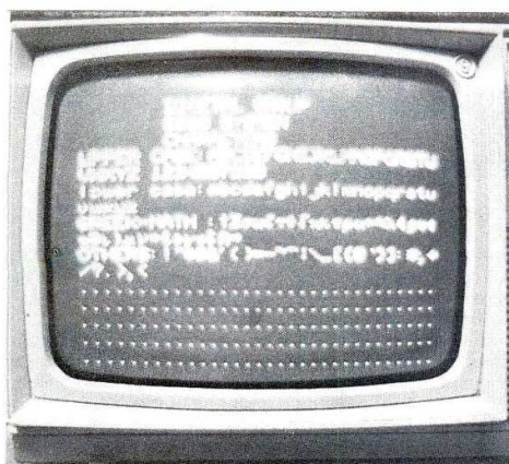
Photo 2. TV Display Showing TV Format and What the Character Generator Will Do.
