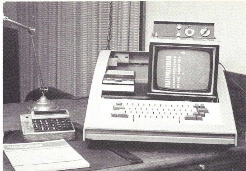
AKIM. Home-brew KIM-1 after TVT-6L and ASCII keyboard are added. Microcomputer, power supplies and keyboard are mounted in surplus KSR 35 enclosure.
