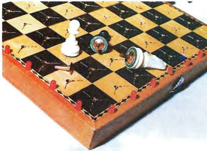
Photo 1: Two pawns, a White Knight, and a loose rivet are shown on top of the electronic chessboard. One row of 8 light emitting diodes (LEDs) is placed along the left side of the board, and another row is placed along the bottom of the board as seen by the human player. Two LEDs are lit to indicate a single square, using an X,Y axis system. A single large hole is drilled in the center of each square to accept entrance of the rivet which is glued to the bottom of each chessman. The rivet completes an electrical circuit between 2 pieces of wire that run from smaller holes through the large central hole. This switching arrangement allows the computer to detect the presence or absence of a piece at each square of the board. In this prototype, an additional set of 3 wires is seen in each square; these wires remain from an earlier, unsuccessful switching attempt.
