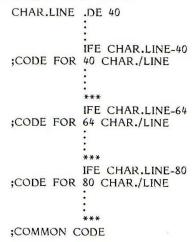
Shown is the arrangement which would assemble code associated with 40 characters per line since CHAR.LINE is defined as equal 40. If you wanted to assemble for 80 characters, simply define CHAR.LINE as equal 80, with SET CHAR.LINE = 80.
