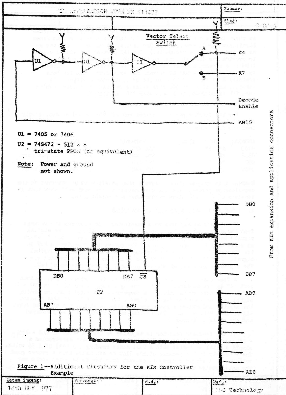
Figure 1--Additional Circuitry for the KIM Controller Example
