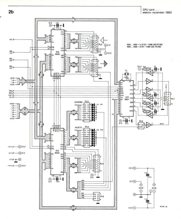
When bipolar ICs are used, power dissipation amounts to 100 mA at  $\pm 12$  V and  $1 \dots 1.5$  A at  $\pm 5$  V. If, however, CMOS circuits are used, current consumption drops to about 100 mA overall, so that it is then possible to supply the CPU from primary cells or rechargeable batteries.
