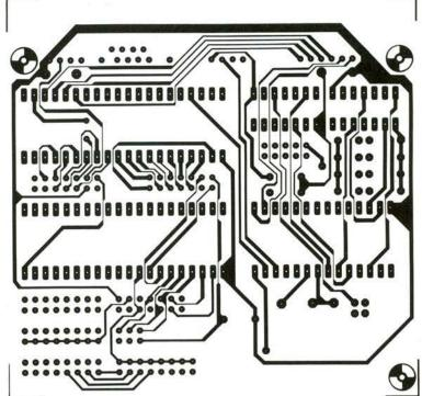
Figure 4. The auxiliary printed circuit board which contains the VIAs and the ACIA.
