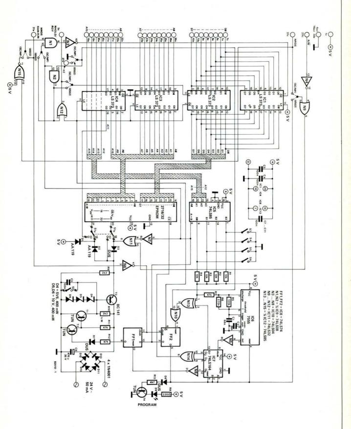
Figure 1. The complete circuit diagram of the 2716/2732 EPROM programmer. The EPROM to be programmed is shown at the centre of the diagram with the latches to the left and the 25 V supply and timing circuitry to the right.
