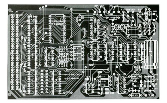
Figure 2. The printed circuit board and component overlay for the programmer.
