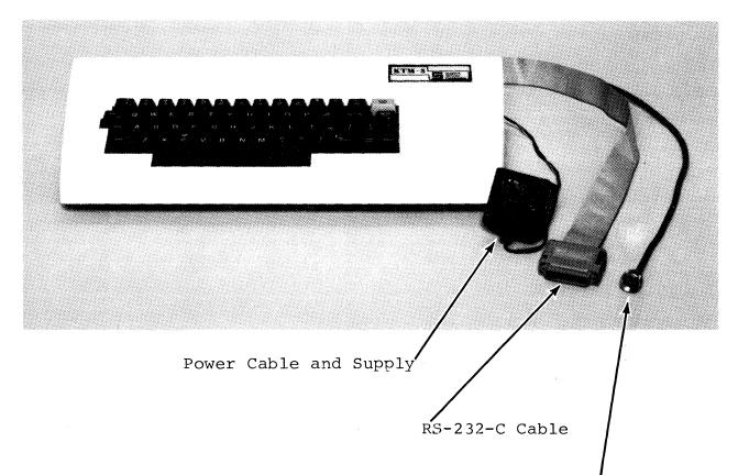
Figure 2-7. KTM-3 Connector Cables
