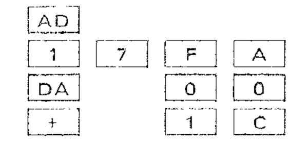
Now, when the NMI interrupt occurs, the program will return to location 1000 and will proceed to save all machine registers before returning control to the operating program.
