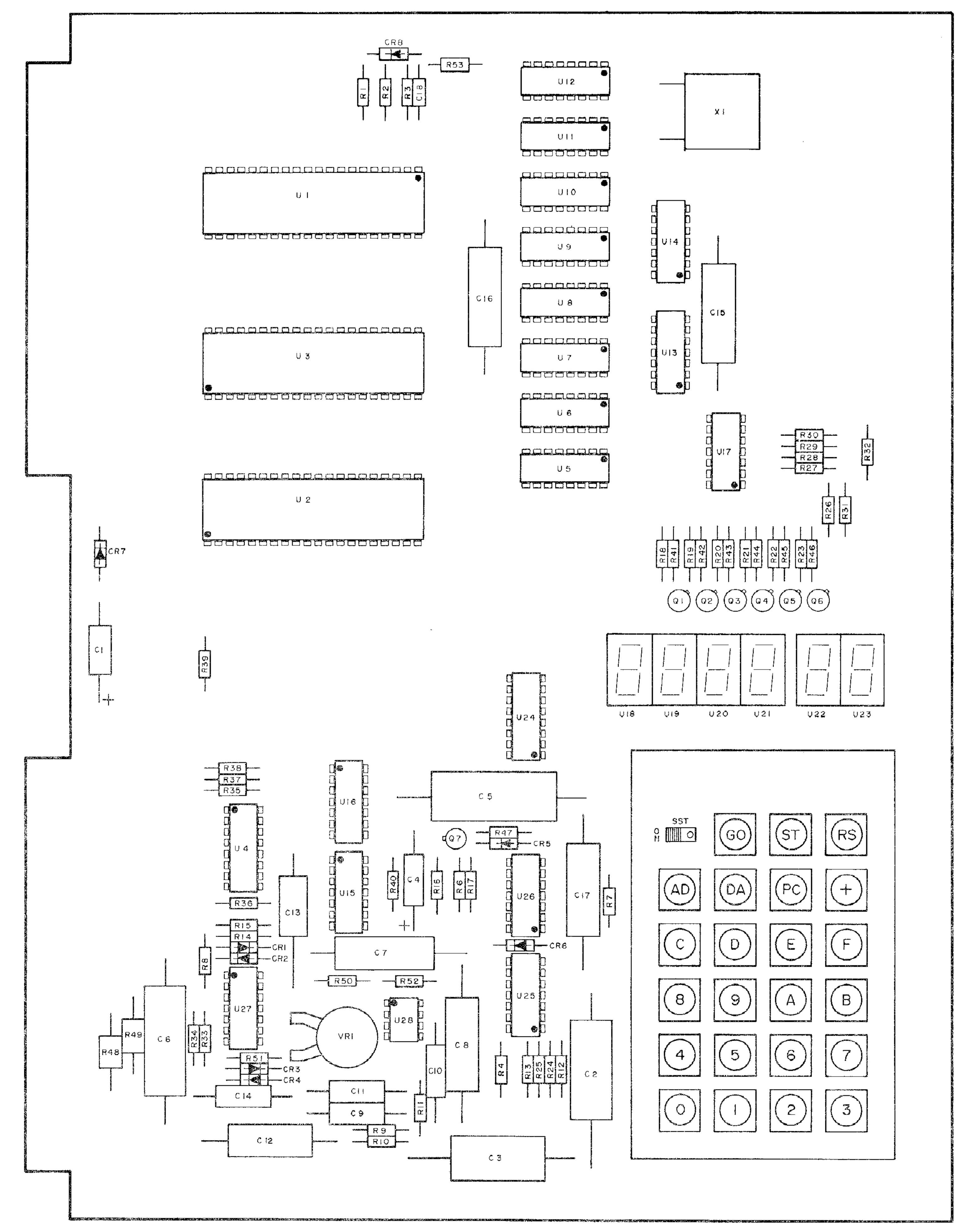
Place the module such that the keyboard is to your lower right and observe that two connector locations extend from the module to your left. The connector area on the lower left is referred to as the Application connector (A). You will note that a 44 pin board edge connector is already installed at this location. The connector area to the upper left is for use by you for future system expansion and is referred to as the Expansion connector (E).
