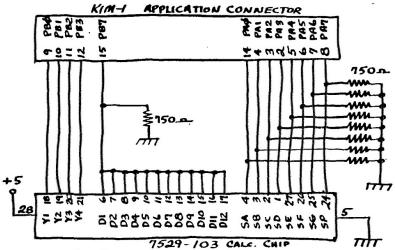
Since the calculator synchronizes all its I/O functions using the digit strobes, so must the computer...
