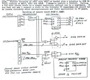
The NOR gate was necessary for the control of the 8T26. Note the negated (inverse) R/W. Also the NOR gates in the RAM-R/W line are not essential but were free. It is not good practice to parallel normal TTL gates, however, where they are on the same substrate, generally, no problems arise. Wired as shown and without the 480 Backplane, direct connection to KIM-1 would provide 9495 to 13TP operation.
