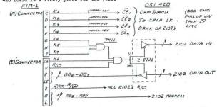
Operation: The 7411 AND gates control the 8726 data buffers such that if any of K9, K5, K6, or K7 are low, the 8726 puts no signal on the data lines to KIM. When KØ, K5, K6, K7 are all high the 8726 direction is controlled by R/W from KIM to read or write to memory selected by any of K1, K2, K3, or K4.
