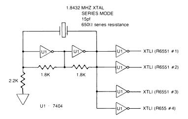
This circuit is identical to the one used on the RM 65 ACIA module and can drive up to two R6551 ACIA devices. To drive more than two XTLI inputs, simply add additional buffering as shown by the dotted lines.
