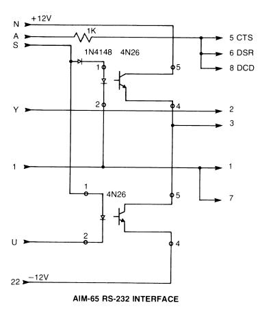
Instead of using another handshake line, the RXD line, pin 2 on the RS-232 connector could be used, since the printer does not have anything to send to AIM, anyway.
