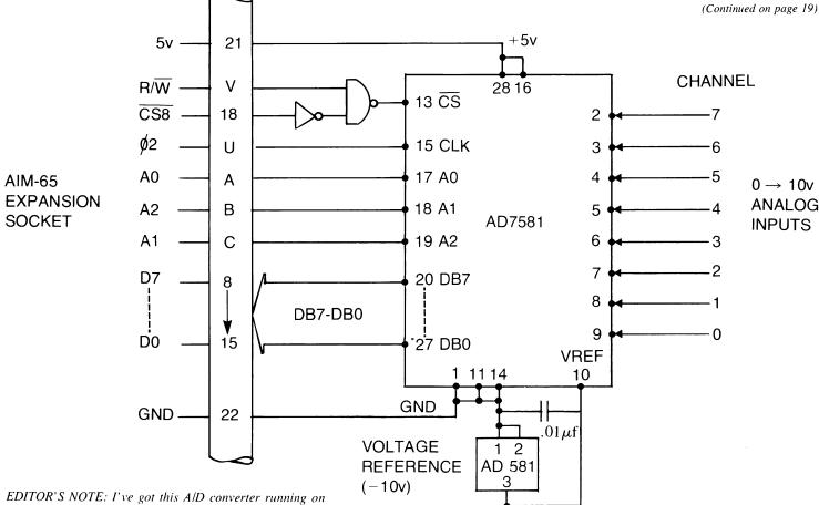
my system and am really impressed with its performance. Just read it like any other memory location and the data is there. No special loops or delays needed. Neato. I took the liberty of modifying Mr. Toomey's program slightly and substituting a voltage reference chip that seemed to be more readily available.
