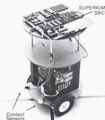
Figure 1. Contact sensors can be mounted around the base of ET-2.
