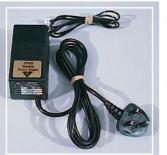
This unit may be used to provide power to a microprocessor board (DT1, DT2 or DT5) and either the DT35 Applications Module or DT34 Input/Output Devices Module.
