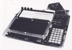
SYM-1 Expansion (E), Application (A) and Auxiliary Application (AA) connectors via one to three SECOND MATEs and 40-conductor ribbon cables. The I/O and bus lines are available at the onboard socket strip. Space is provided for up to three additional socket strips. The FIRST MATE is electrically compatible with the KIM-1\* and AIM-65\* microcomputers.
