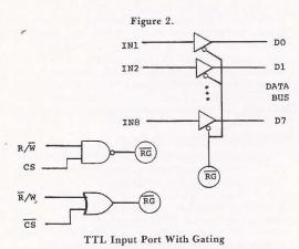
If read gate signals are required for several ports, a single three to eight decoder chip can be used to get eight read gates from a coarser select. The R/W line is used as an enable and is internally gated with all the outputs, as shown in figure 3.
