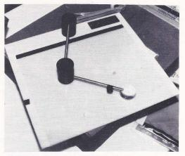
For low-cost digital input (about \$200), how about this? Your Apple (or whatever) simply reads the position of the two pots which are mounted in the pivot points to compute the position of the arm. Clever, huh???
