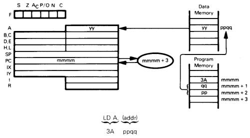
Load the contents of the memory byte (addressed directly by the second and third bytes of the LD A, (addr) instruction object code) into the Accumulator. Suppose memory byte  $084A_{16}$  contains  $20_{16}$ . After the instruction
