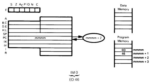
This instruction places the CPU in interrupt mode 0. In this mode, the interrupting device will place an instruction on the Data Bus and the CPU will then execute that instruction. No registers or statuses are affected.
