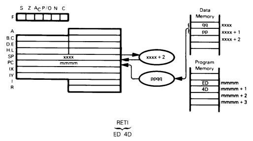
Move the contents of the top two stack bytes to the Program Counter; these two bytes provide the address of the next instruction to be executed. Previous Program Counter contents are lost. Increment the Stack Pointer by 2, and address the new top of stack.
