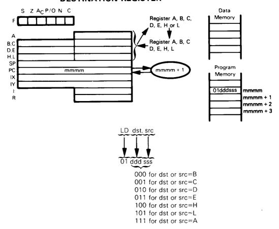
The contents of any designated register are loaded into any other register.
