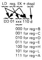
Load specified register from memory location (specified by the sum of the contents of the IX register and the displacement digit d).
