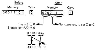
This instruction is identical to RR (IY+disp), but uses the IX register instead of the IY register.
