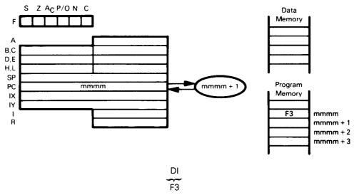
When this instruction is executed, the maskable interrupt request is disabled and the INT input to the CPU will be ignored. Remember that when an interrupt is acknowledged, the maskable interrupt is automatically disabled.
