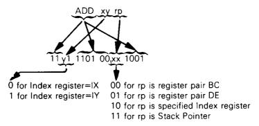
Add the contents of the specified register pair to the contents of the specified Index register.
