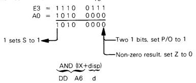
This instruction is identical to AND (IY+disp), except that it uses the IX register instead of the IY register.
