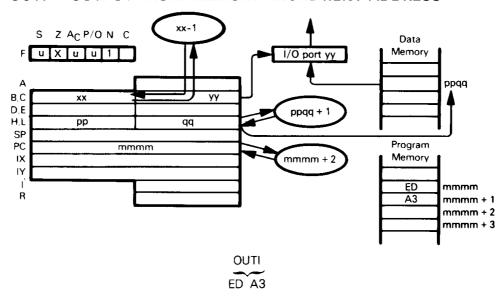
Output from memory location specified by HL to I/O port addressed by Register C. Register B is decremented and the HL register pair is incremented.
