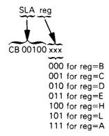
Shift contents of specified register left one bit, resetting the least significant bit to 0. Suppose Register B contains 1F<sub>16</sub>, and Carry=1. After execution of
