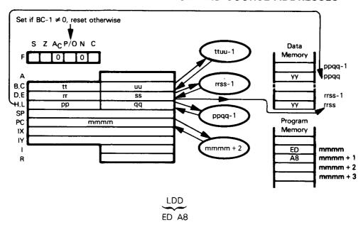
Transfer a byte of data from memory location addressed by the HL register pair to memory location addressed by the DE register pair. Decrement contents of register pairs BC, DE, and HL.
