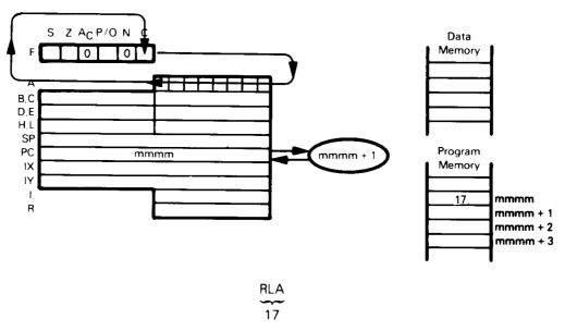
Rotate Accumulator contents left one bit through Carry status.
