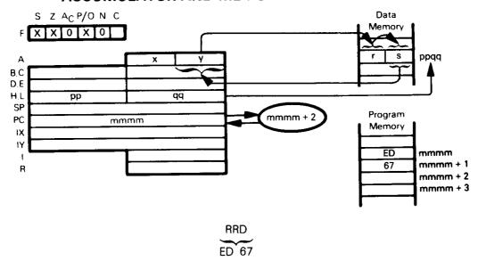
The four high-order bits of a memory location (specified by the contents of register pair HL) are copied into the four low-order bits of the same memory location. The previous contents of the four low-order bits are copied into the four low-order bits of the Accumulator. The previous four low-order bits of the Accumulator are copied into the four high-order bits of the specified memory location.
