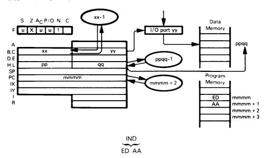
Input from I/O port (addressed by Register C) to memory location (specified by HL). Decrement Registers B and HL.
