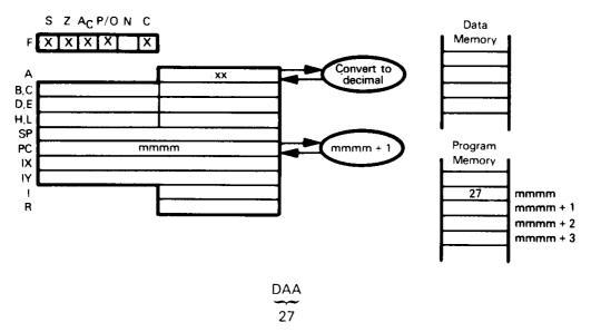
Convert the contents of the Accumulator to binary-coded decimal form. This instruction should only be used after adding or subtracting two BCD numbers; i.e., look upon ADD DAA or ADC DAA or INC DAA or SUB DAA or SBC DAA or DEC DAA or NEG DAA as compound, decimal arithmetic instructions which operate on BCD sources to generate BCD answers.
