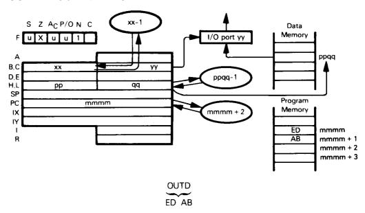
Output from memory location specified by HL to I/O port addressed by Register C. Registers B and HL are decremented.
