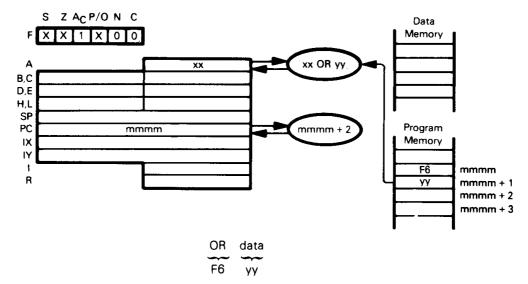
OR the Accumulator with the contents of the second instruction object code byte. Suppose  $xx=3A_{16}$ . After the instruction
