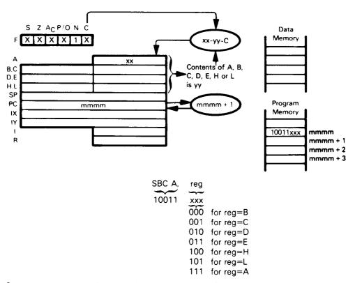
Subtract the contents of the specified register and the Carry status from the Accumulator.
