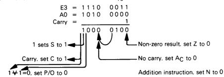
The ADC instruction is most frequently used in multibyte addition for the second and subsequent bytes.
