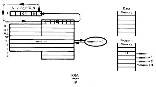
Rotate Accumulator contents right one bit through Carry status.
