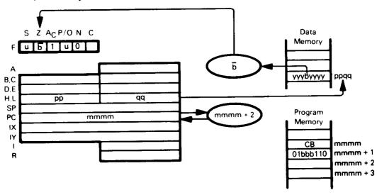
The illustration shows execution of BIT 4,(HL). Bit 0 is the least significant bit.
