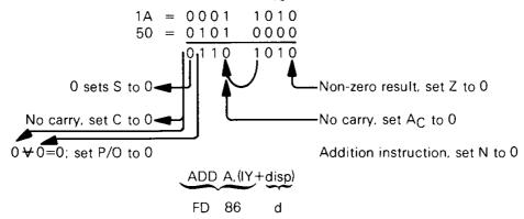
This instruction is identical to ADD A.(IX+disp), except that it uses the IY register instead of the IX register.
