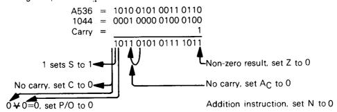
The ADC instruction is most frequently used in multibyte addition for the second and subsequent bytes.
