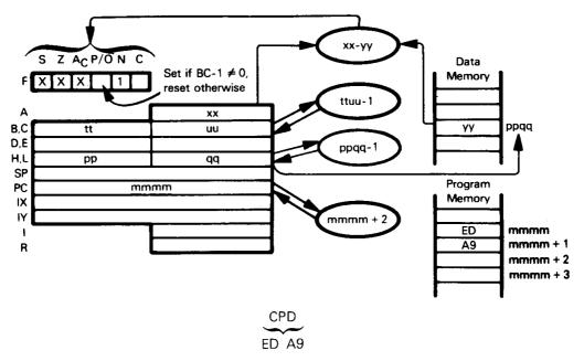
Compare the contents of the Accumulator with the contents of memory location (specified by the HL register pair). If A is equal to memory, set Z flag. Decrement the HL and BC register pairs. (BC is used as the Byte Counter.)
