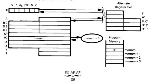
The two-byte contents of register pairs AF and A'F' are exchanged. Suppose AF contains  $4F99_{16}$  and A'F' contains  $10AA_{16}$ . After execution of EX AF AF'
