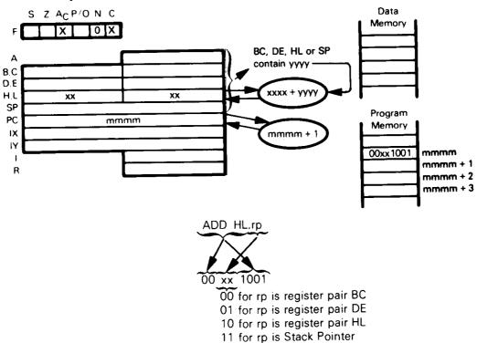
Add the 16-bit value from either the BC, DE, HL register pair or the Stack Pointer to the HL register pair.
