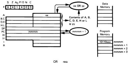
Logically OR the contents of the Accumulator with the contents of Register A, B, C, D, E, H or L. Store the result in the Accumulator.
