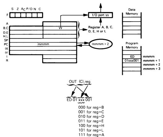
Suppose yy=1F $_{16}$  and the contents of H are AA $_{16}$ . After the execution of OUT (C),H
