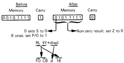
This instruction is identical to RL (IX+disp), but uses the IY register instead of the IX register.
