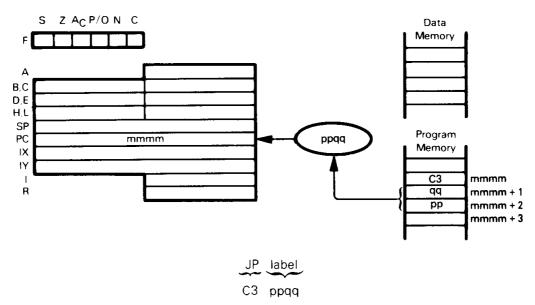
Load the contents of the Jump instruction object code second and third bytes into the Program Counter; this becomes the memory address for the next instruction to be executed. The previous Program Counter contents are lost.
