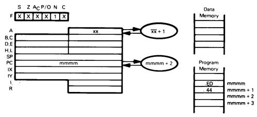
Negate contents of Accumulator. This is the same as subtracting contents of the Accumulator from zero. The result is the two's complement. 80H will be left unchanged.
