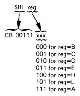
Shift contents of specified register right one bit. Most significant bit is reset to 0.
