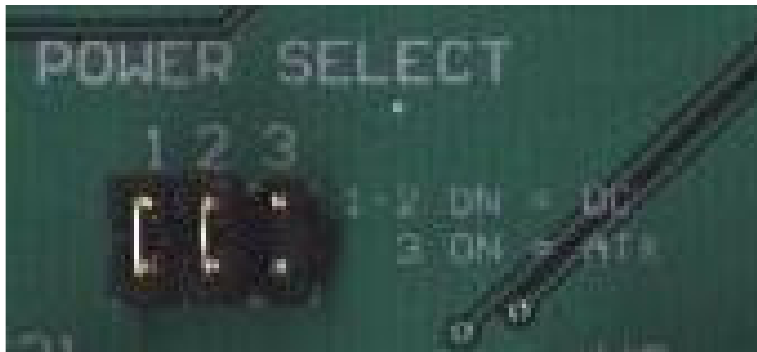
Figure 5: Jumper Select 1-3 shown ready for DC wall brick (not included)
