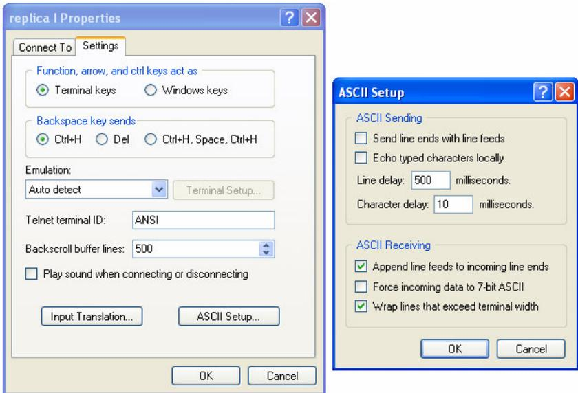
Figure 13: ASCII settings for COM port
