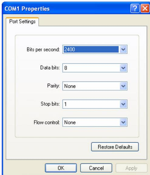
Figure 11: Proper serial port settings
