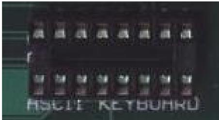
**Figure 6: ASCII keyboard port**
