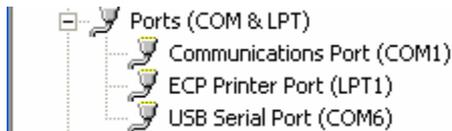
**Figure 7: Device Manager showing new USB Serial Port**
