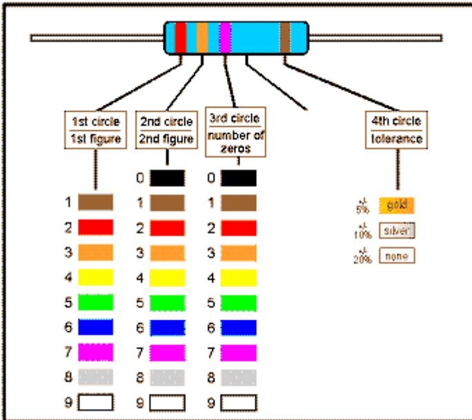
Figure 8: Resistor color code chart
