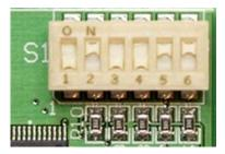
Figure 2: Typical dip switch configuration for the Apple1 and Replica1 computers.
