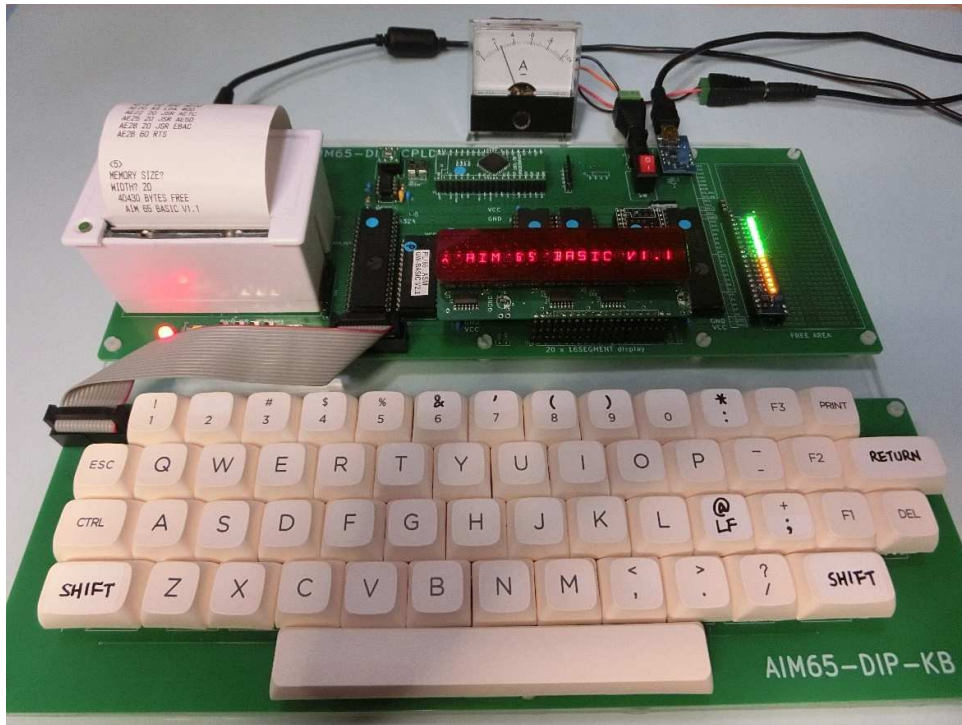
Reproduction AIM65-DIP-CPLD with 5V operation
