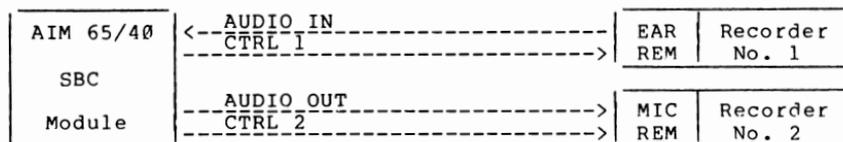
d. Two recorders with two remote control lines
