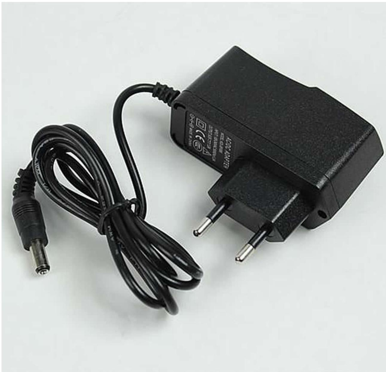
The center pin is positive. The outer is GND.
