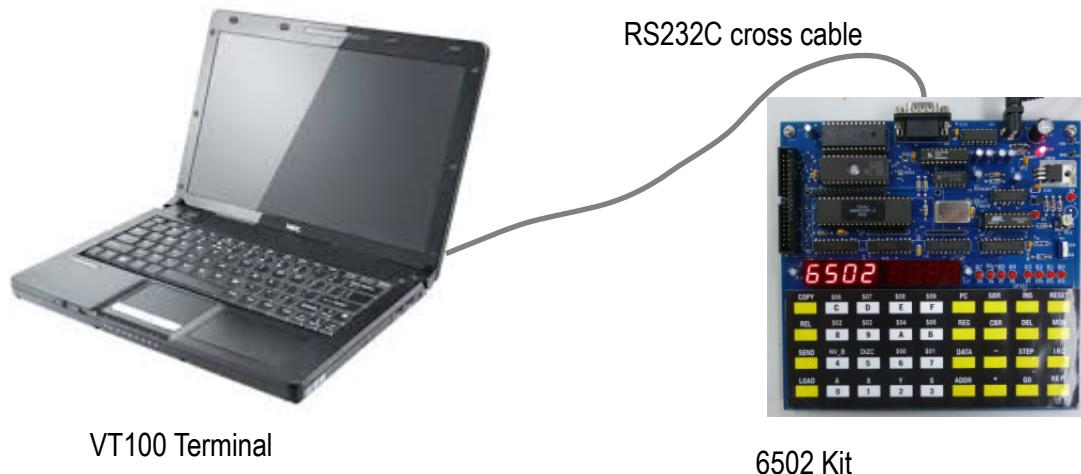
The example shows connecting the laptop with COM1 port to the RS232C port. New laptop has no COM port, we may use the USB-RS232 adapter for converting the USB port to RS232 port.
