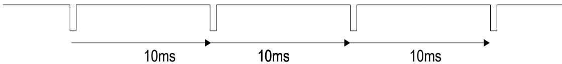
The 10ms tick signal measured at P3.7 pin.
