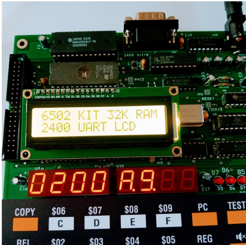
**Note: Insert/Remove the LCD module must be done when the kit is powered off.**
