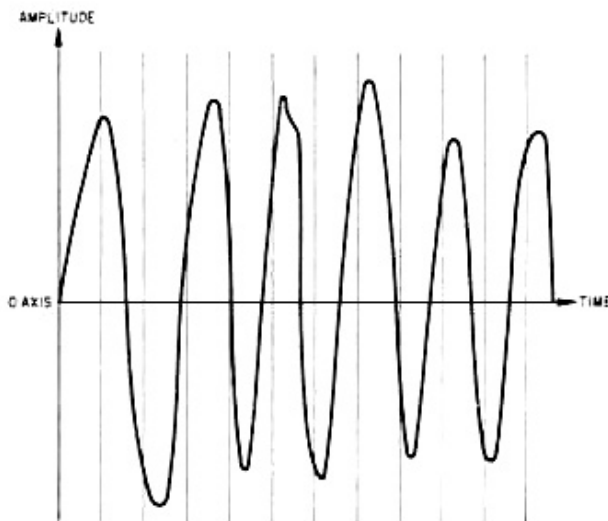
Fig. 7-3. High pass filter output.
