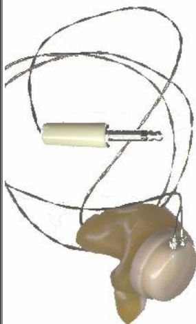
Top: Special ear mold to receive auditory suggestions from the blackjack computer.
